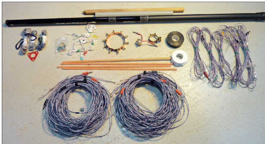
Figure 6 — Entire antenna kit laid out. At the top: sharpened support stake that is driven into the ground; \frac{3}{4} inch PVC pipe sleeve that slides over support stake; 16 foot, five-section telescopic Shakespeare® Wonderpole. Under the Wonderpole from left to right: backup red guy ring with three guy line sets comprised of miniature carabiner, 10 feet of guy string, and plastic bag to hold rocks to anchor guy string; bag of rubber bands; color-coded radiator support strings; copper ground ring; SO-239 feed point; radiator feed ring; electrical tape to back up tired Wonderpole friction joints; five radiator lines with captive wire guides on the four outboard lines. At the center and bottom: four spreader arms that fit into the white PVC spreader hub; 16 sets of ground radials, each secured with a hook-and-loop strap.
