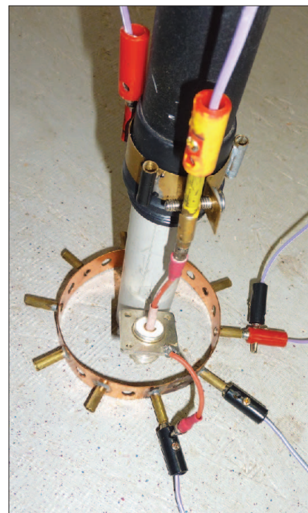
Figure 5 — Bottom of antenna showing radiator feed ring clamped to end of five section telescopic fiberglass fishing pole that slides onto 1/4 inch PVC pipe sleeve that slips over supporting stake driven into ground. The center conductor of the SO-239 feed point plugs into the bottom of the feed ring and the shell is connected to the ground ring. Connections are doubled up by using banana plugs with an auxiliary socket. Ground and feeder ring banana sockets are shop-fashioned from 3/16 inch OD brass tubing.
