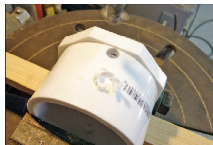
Figure 4 — Drilling hole through PVC bushing to form the hub for the spreader arms. Excess material on the spreader hub was later cut off to reduce its size.
